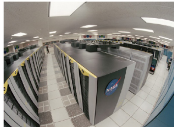
NASA/Ames Columbia machine—a 10240 processor SGI Altix system.
