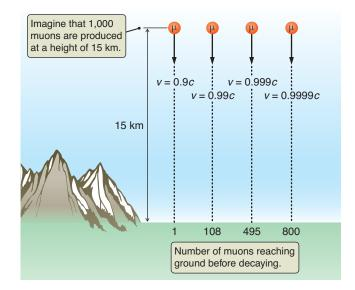
**FIGURE 18.6** Muons created by cosmic rays high in Earth's atmosphere would decay long before reaching the ground if they were not traveling at nearly the speed of light. An observer on the ground sees a longer muon lifetime because of time dilation. Here we show what happens to four different sets of 1,000 muons produced at an altitude of 15 km for a variety of speeds.
