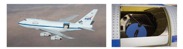
FIGURE 6.27 SOFIA is a 2.5-meter infrared telescope that is mounted in a Boeing 747 aircraft.
