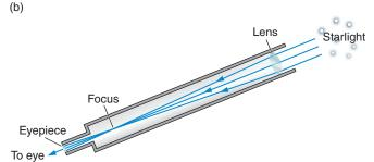
**FIGURE 6.4** The Yerkes 1-meter refractor uses a lens to collect light. The parts of a refractor are sketched in (b).
