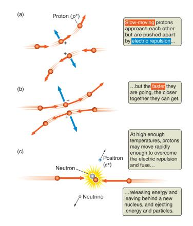
**FIGURE 14.3** Atomic nuclei are positively charged and so repel each other. (a, b) If two nuclei are moving toward each other, the faster they are going, the closer they will get before veering away. (c) At the temperatures and densities found in the centers of stars, thermal motions of nuclei are energetic enough to overcome this electric repulsion, so fusion takes place.
