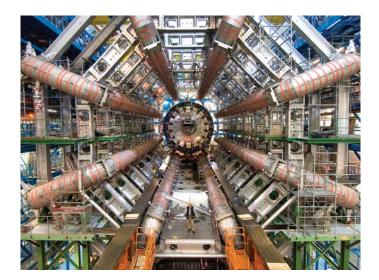
**FIGURE 6.32** The ATLAS particle detector at CERN's Large Hadron Collider near Geneva, Switzerland. The enormous size of this instrument is evident from the person standing near the bottom center of the picture.
