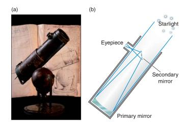
**FIGURE 6.5** Newton's reflecting telescope. The parts of a reflector are sketched in (b).
