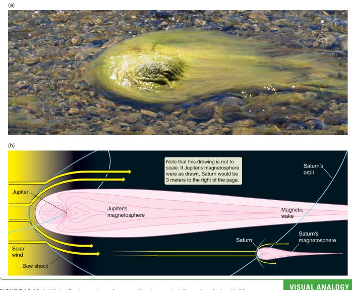
FIGURE 10.19 (a) Water flowing past a rock sweeps the algae against the rock and into a "tail," or wake, pointing in the direction of the water's flow. (b) The solar wind compresses Jupiter's (or any other) magnetosphere in the direction toward the Sun and draws it out into a magnetic wake in the direction away from the Sun. Jupiter's wake stretches beyond the orbit of Saturn.
