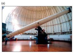
Yerkes: 1-meter-diameter lens World's largest refracting telescope
