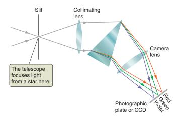
FIGURE 6.21 A diagram of a prism spectrograph.
