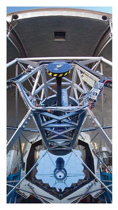
**FIGURE 6.12** Each of the Keck 10-meter reflectors uses an aligned group of 36 hexagonal mirrors to collect light.
